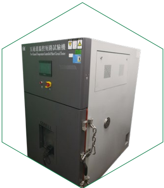
Short circuit Test
